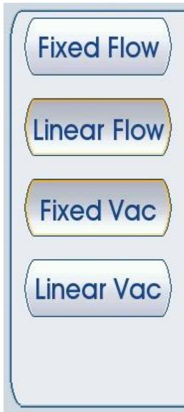
**Linear Flow:** When position (2) is reached, the peristaltic pump speed, or Flow (cc/min), is controlled by the actuation of the foot pedal between zero and the maximum limit set by the user using the UP or DOWN arrow keys or the default setting of the Flow parameter.
