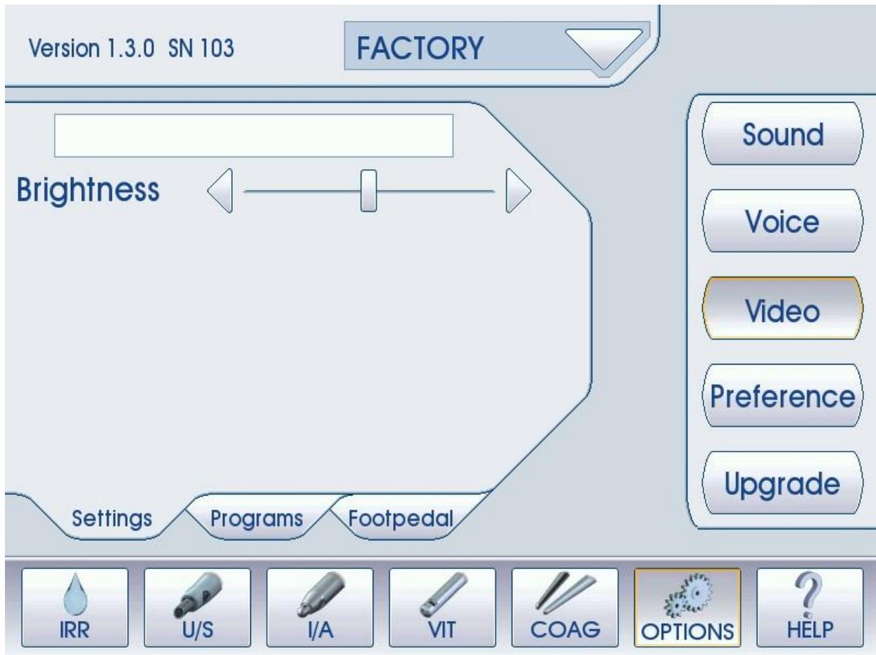
The Video mode allows the user to set their preferences for the LCD display brightness.
