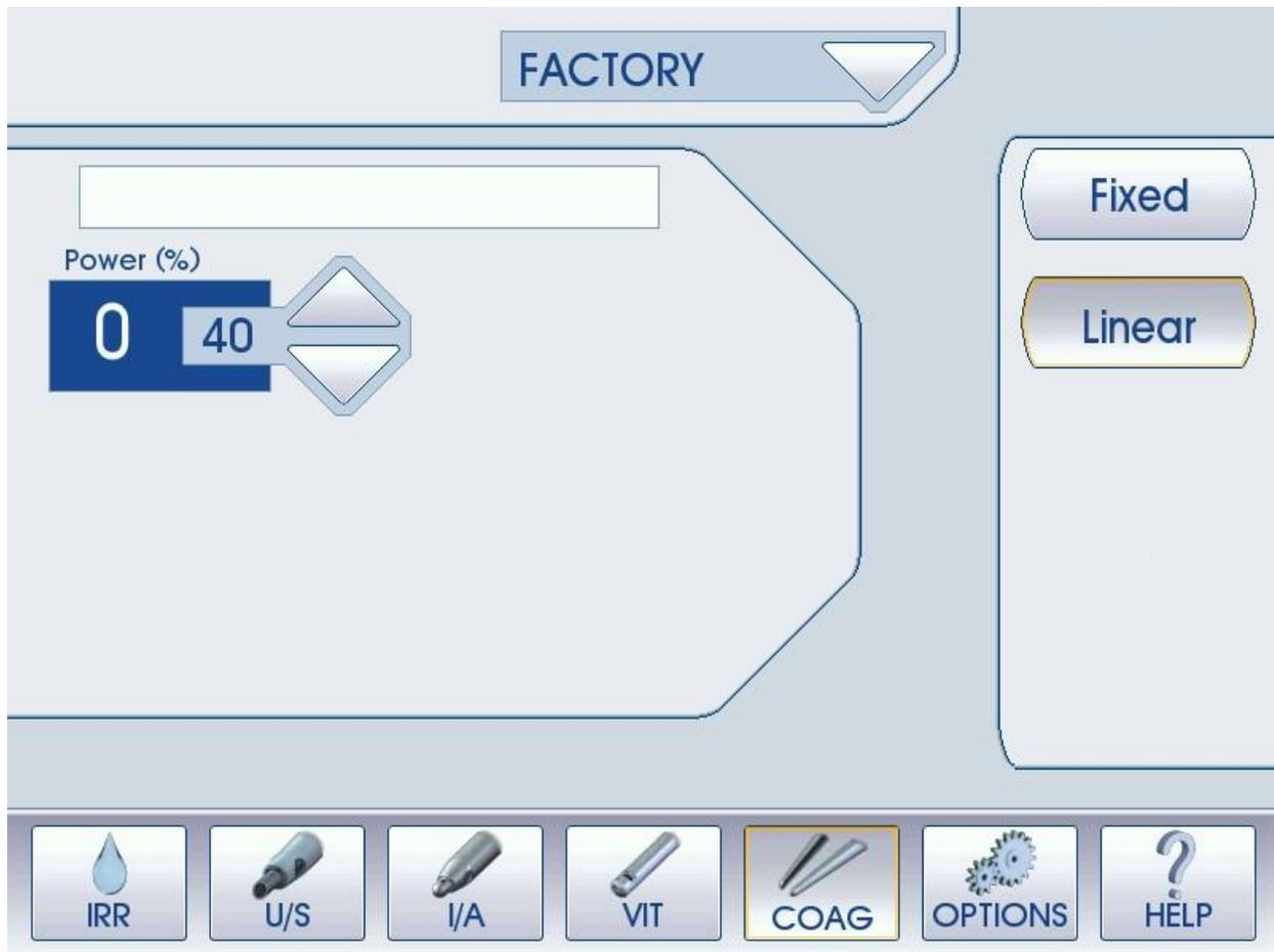
The Coagulation mode is mainly used for cauterizing small blood vessels. Most surgeons use the bipolar coagulation for this function. An isolated 315 kHz frequency cautery circuit allows for non-contact tissue coagulation.
