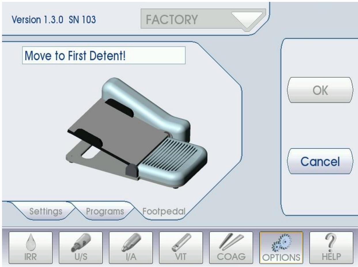
The Model 3000 comes pre-calibrated with the foot pedal included in the original system package. However, the foot pedal can be recalibrated at any time to the three (3) foot pedal positions you desire.
