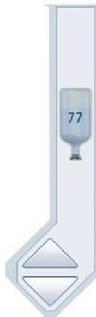
The arrow keys can also be pressed and held to move the solution container to a desired height, and then pressed to obtain the exact height.
