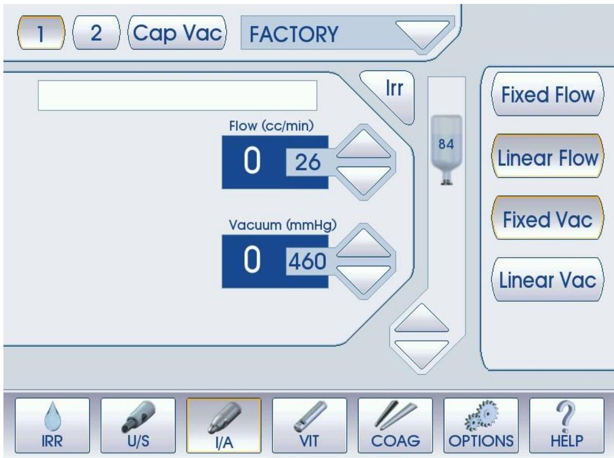
Control of the irrigation pinch valve, venting pinch valve, and peristaltic pump is accomplished by actuation of the foot pedal.
